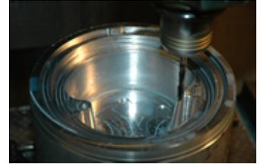
Fidelity started with two OKK vertical machining centers, a 1990-model MCV820 and a smaller PCV55 from 1996. "We needed maximum efficiency from them, primarily to keep up with cable-over-molding demand," he says. "Mechanically, these machines were capable of moving at 300 to 400 inches per minute, but the CNC controllers are incapable of pushing the machines accurately at anywhere near these speeds."
