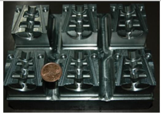
A larger mold with more open areas would be much simpler to program. “This is machining with almost no clearance for the cutter,” Litster points out, “so extremely precise control of all cutter movement is essential.”
